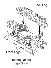
Figure 19 - Installing Front and Back Logs (Number and Style of Logs May Vary)
